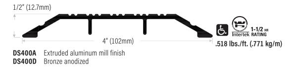
Thresholds are supplied with punched countersunk holes with screws and plugs and are only available in the following NET lengths: 36-1/2" (927mm), 49" (1245mm), 73" (1854mm), 110" (2794mm), 147" (3734mm)
