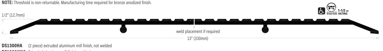
**DS1300HWA** Extruded aluminum mill finish, welded
