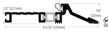
**DS276TBAT** Extruded aluminum mill finish with vinyl thermal break insert & TPE (T) insert
