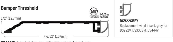
**DS444AV** Extruded aluminum mill finish with vinyl insert, grey **DS444DV** Bronze anodized
