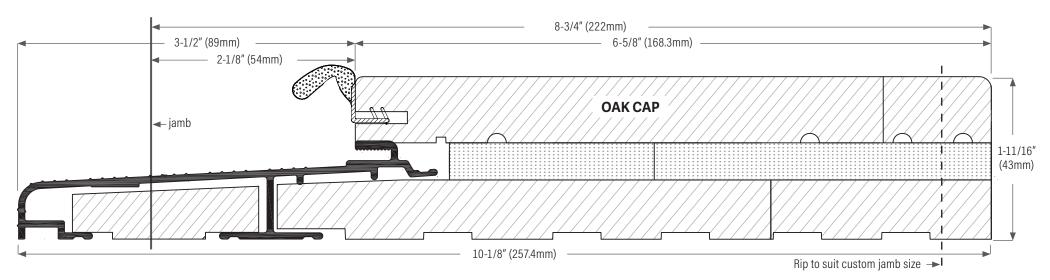
**DS1018A0AK150** Extruded aluminum sill, mill finish with oak cap, 10-1/8" (257mm) x 150" (3810mm) length. **DS1018D0AK150** Extruded aluminum sill, bronze anodized with oak cap, 10-1/8" (257mm) x 150" (3810mm) length.
