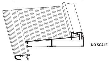
Sill extension eliminates the time consuming notching on regular sill. Snap & screw sill extension to sill. You choose the length of the sill horns.
