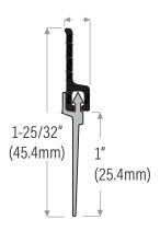
**DS140AV** Extruded aluminum mill finish with vinyl insert, grey
