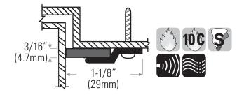
**DS142CN** Extruded aluminum clear anodized with neoprene insert
