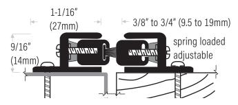
**DS151C** Extruded aluminum clear anodized (no pile insert). Sold in single units, order 2 lengths for meeting stile. **DS151CP** Clear anodized with polypropylene pile insert.
