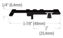
**DS185CP** Extruded aluminum clear anodized with pile insert **DS185DP** Bronze anodized
