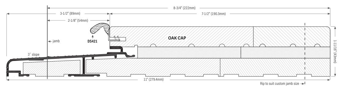
**DS2111A0AK150** Extruded aluminum sill, mill finish with oak cap, 11" (279mm) x 150" (3810mm) length. **DS2111D0AK150** Extruded aluminum sill, bronze anodized with oak cap, 11" (279mm) x 150" (3810mm) length.
