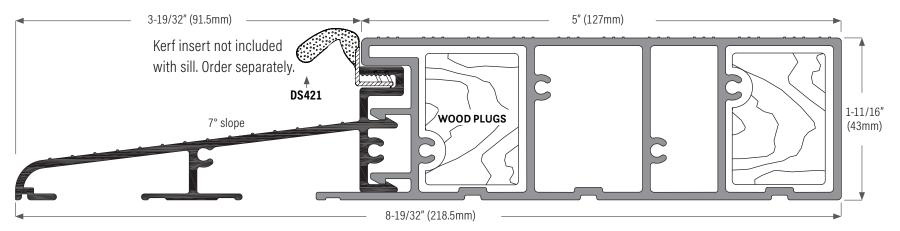
**DS2858AVT150** Extruded aluminum sill mill finish with PVC interior cap tan & 3 wood inserts. 150" (3810mm) length.
