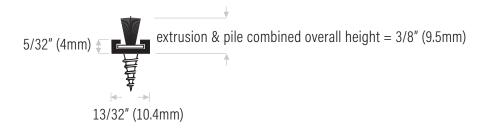
**DS369A7535G** Aluminum extrusion mill finish with fin pile insert, grey
