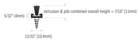
**DS369A7540G** Aluminum extrusion mill finish with fin pile insert, grey
