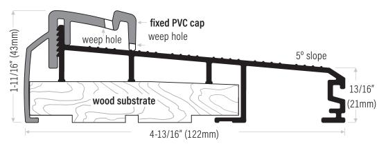
**DS459AVBL**Extruded aluminum sill, mill finish with wood substrate & fixed PVC cap, black**DS459AVT**Extruded aluminum sill, mill finish with wood substrate & fixed PVC cap, tan**DS459AVW**Extruded aluminum sill, mill finish with wood substrate & fixed PVC cap, white
