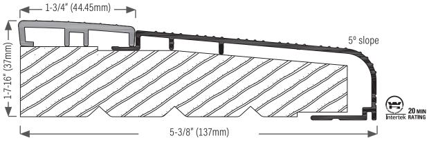
**DS512AVT** Extruded aluminum sill, mill finish with fixed vinyl cap, tan. **DS512DVBL** Bronze anodized with fixed PVC cap, black.
