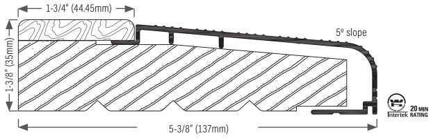
DS512AOAK Extruded aluminum sill mill finish with fixed oak cap
