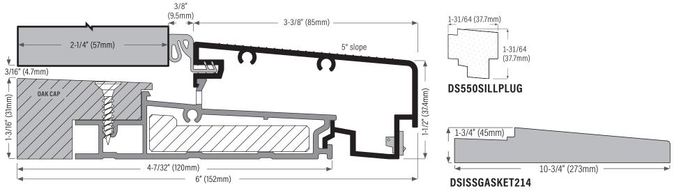
DS552A2OAK Mill finish with oak cap for 2-1/4" (57mm) door thickness
