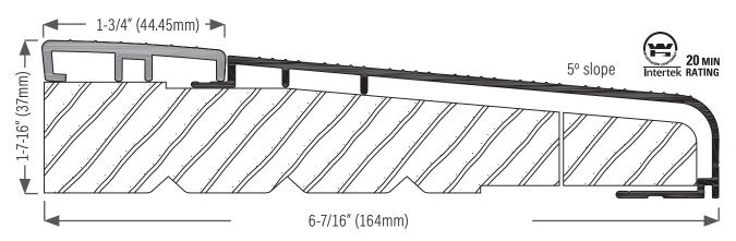
**DS612AVT** Extruded aluminum sill, mill finish with fixed PVC cap, tan.
