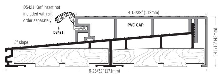
**DS657AVW** Extruded aluminum sill, mill finish with interior fixed PVC cap, white
