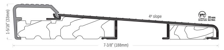
DS738AVT Extruded aluminum sill, mill finish with fixed PVC cap, tan
