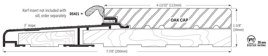
DS778AOAK Extruded aluminum sill, mill finish with interior oak cap. Length available: 150" (3810mm) only
