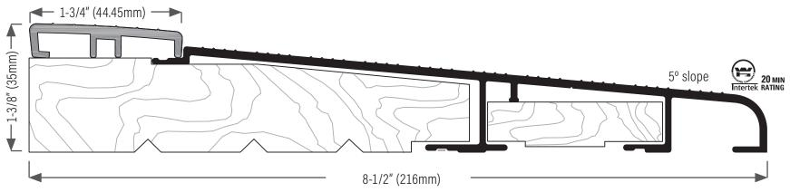
**DS812AVT** Extruded aluminum sill, mill finish with fixed PVC cap, tan.
