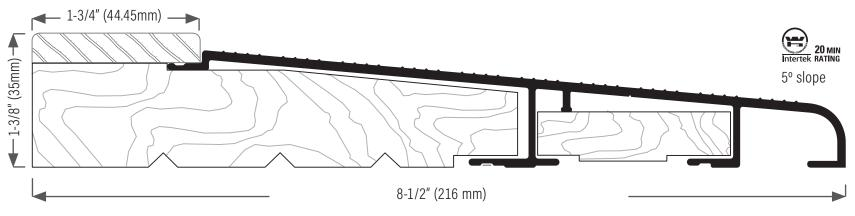
**DS812AOAK** Extruded aluminum sill, mill finish with fixed oak cap. **DS812DOAK** Bronze anodized with fixed oak cap.
