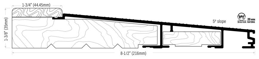
**DS814AOAK** Extruded aluminum sill, mill finish with fixed oak cap. Length available: 108" (2743mm) only **DS814DOAK** Bronze anodized with fixed oak cap.
