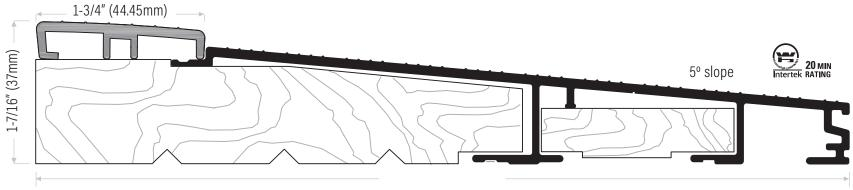
**DS814AVT** Extruded aluminum sill, mill finish with fixed PVC cap, tan. Length available: 108" (2743mm) only **DS814DVBL** Bronze anodized with fixed PVC cap, black.
