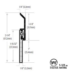
DS138C-2 Extruded aluminum clear anodized with rubber insert, black, 1/8" x 2" (3.2mm x 51mm) DS138D-2 Bronze Anodized
