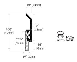
**DS138C** Extruded aluminum clear anodized with rubber insert, black, 1/8" x 1-3/8" (3.2mm x 35mm) **DS138D** Bronze anodized
