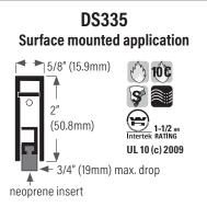
WARNING: Do not pull drop bar out of case unless disengaged from spring or damage will occur and void warranty
