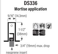
WARNING: Do not pull drop bar out of case unless disengaged from spring or damage will occur and void warranty
