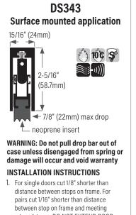
between stop on frame and meeting edge of door. - DO NOT EXTEND DROP BAR WHILE CUTTING. Insert (2) nails provided into the small holes on the side of the drop bar to keep drop bar extended while cutting. Do not cut from end with adjusting rod. **Maximum cut door bottoms** 25" to 35" (635mm to 890mm) = 2" (£12mm)
