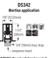
WARNING: Do not pull drop bar out of case unless disengaged from spring or damage will occur and void warranty
