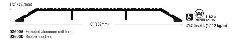
Thresholds are supplied with punched countersunk holes with screws and plugs and are only available in the following NET lengths: 36-1/2" (927mm), 49" (1245mm), 73" (1854mm), 110" (2794mm), 147" (3734mm)
