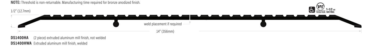
Wide threshold is standard punched or drilled unless otherwise specified and is available in the following NET lengths: 36-1/2" (927mm), 49" (1245mm), 73" (1854mm), 110" (2794mm), 147" (3734mm).
