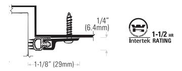
**DS100AT** Extruded aluminum mill finish with TPE (T) insert
