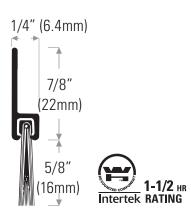
**DS148CNB** Extruded aluminum clear anodized with nylon brush insert **DS148DNB** Bronze anodized with nylon brush insert **DSBRUSH58BL** Replacement brush insert, black
