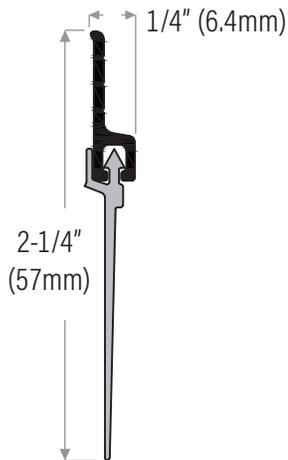
**DS156AV** Extruded aluminum mill finish with vinyl insert, grey
