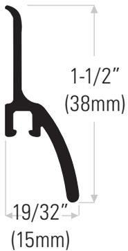
**DS164A** Extruded aluminum mill finish. Lengths available: 36" (914mm) & 48" (1219mm)
