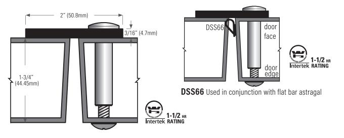
**DS184SSATIN** Flat bar, **STAINLESS STEEL**. Lengths available: 84" (2134mm), 96" (2438mm), 144" (3658mm) **DS188-2PS** Flat bar, **STEEL** prime coated 2" (51mm) wide. Lengths available: 84" (2134mm), 96" (2438mm), 144" (3658mm)
