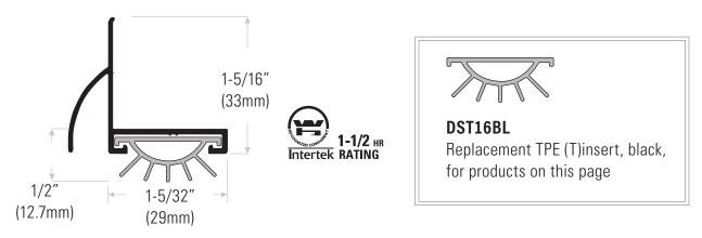
**DS210AT** Extruded aluminum mill finish with TPE (T) insert **DS210DT** Bronze anodized
