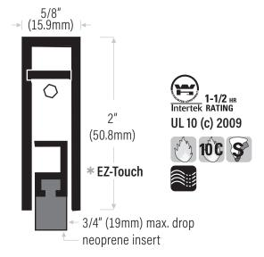
**DS335CN** Extruded aluminum clear anodized with neoprene insert, black **DS335DN** Bronze anodized with neoprene insert, black. Custom order, call for manufacturing time. 36" & 48" only (914mm & 1219mm)
