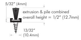
DS369A7545G Aluminum extrusion mill finish with fin pile insert, greyDS369A7445W Aluminum extrusion mill finish with fin pile insert, whiteDS369A7145B Aluminum extrusion mill finish with fin pile insert, black
