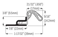
DS422B Extruded aluminum painted brown with gasket insert, brownDS422C Clear anodized with black gasket insertDS422W Painted white with white gasket insert
