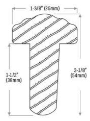
DS196P80M1 1-3/8" (35mm) primed fir, machined for flush bolts, top only. 80" (2032mm)
