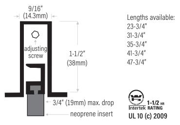
**DS386AN24** Extruded aluminum mill finish with neoprene insert, black **DS386AN32** Extruded aluminum mill finish with neoprene insert, black **DS386AN36** Extruded aluminum mill finish with neoprene insert, black **DS386AN42** Extruded aluminum mill finish with neoprene insert, black **DS386AN48** Extruded aluminum mill finish with neoprene insert, black
