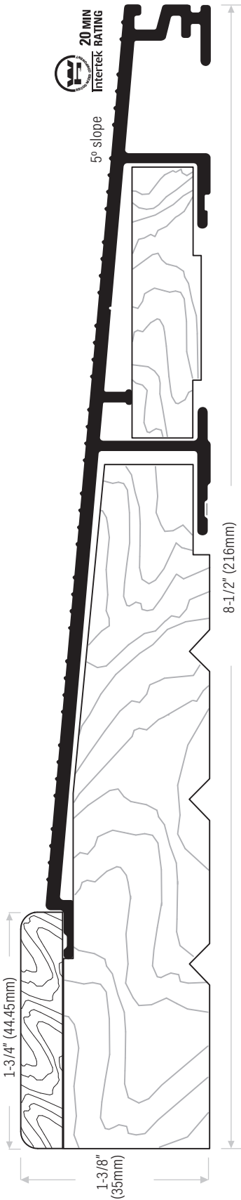
DS814A0AK Extruded aluminum sill, mill finish with fixed oak cap. Length available: 108" (2743mm) only DS814DOAK Bronze anodized with fixed oak cap.
