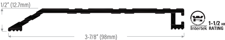
DS444A Extruded aluminum mill finish DS444D Bronze anodized
