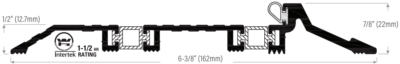
DS277X6TBAT Mill finish with vinyl thermal break & TPE (T) insert, black (rated)
