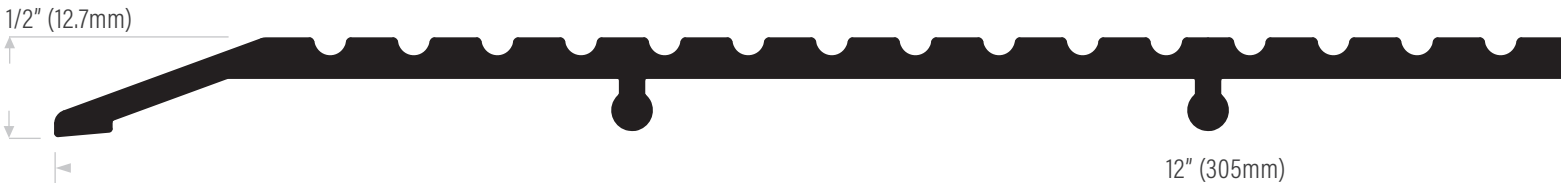
DS1200HC (1 piece) extruded aluminum clear anodized
