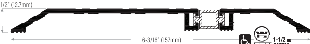
DS602TBA Extruded aluminum mill finish with vinyl thermal break
