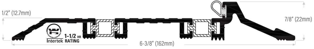
DS277X6TBAT Mill finish or black anodized with vinyl thermal break & TPE (T) insert, black (rated)
