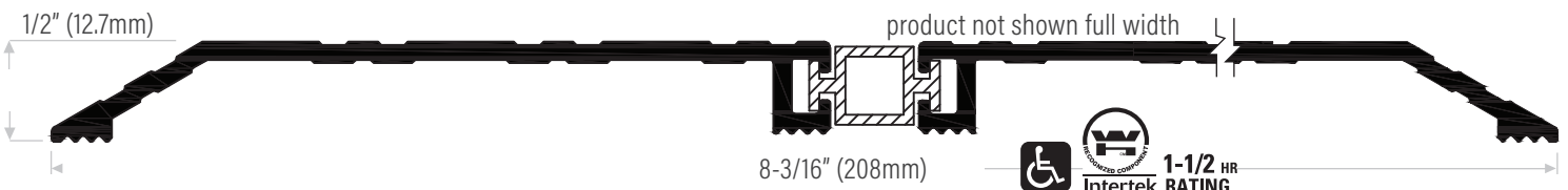
DS801TBA Extruded aluminum mill finish or black anodized with vinyl thermal break
