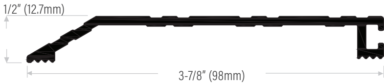
DS444A Extruded aluminum mill finish DS444D Black anodized
