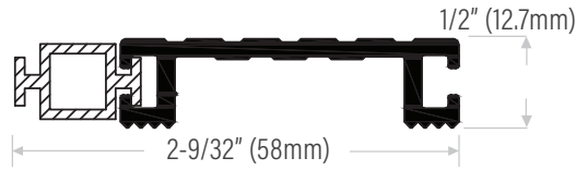
DS202TBA Extruded aluminum mill finish or black anodized with thermal break insert
