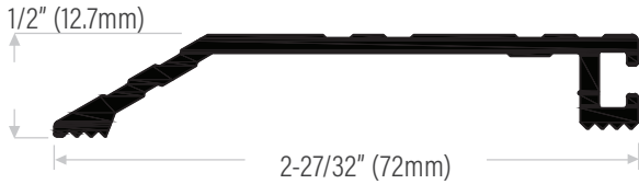
DS333A Extruded aluminum mill finish DS333D Black anodized
