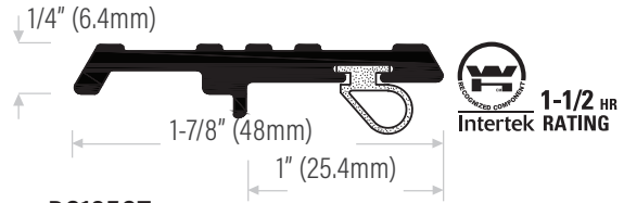
DS185CT Extruded aluminum clear anodized with TPE (T) insert DS185DT Black anodized
