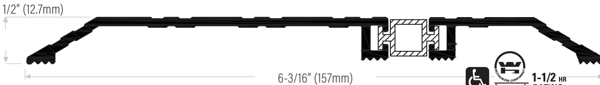
DS602TBA Extruded aluminum mill finish or black anodized with vinyl thermal break
