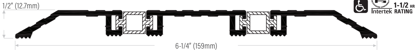
DS603TBA Extruded aluminum mill finish or black anodized with 2 thermal breaks
